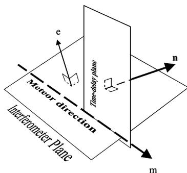
Fig. 2. The line containing the meteor directions is the intersection of the “interferometer plane” determined from the echo direction and the “time-delay plane” determined from the time delays of the echoes on the remote stations relative to the main station.
