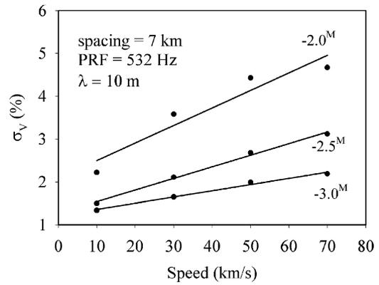
Fig. 5. Results of numerical simulation for determining the fraction of echoes that will yield orbits as a function of speed magnitude of the train relative to that which is just detectable at the main station. Spacing = 7 km; PRF = 532 Hz.
