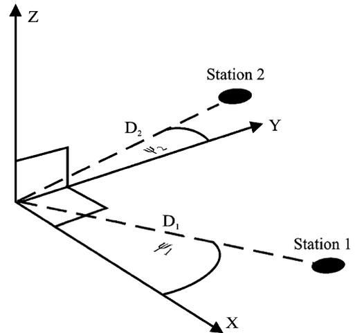
Fig. 3. Definition of the angles  $\psi_1$  and  $\psi_2$  involved when the vectors from the main to the remote stations are not aligned with the axes of the coordinate system.
