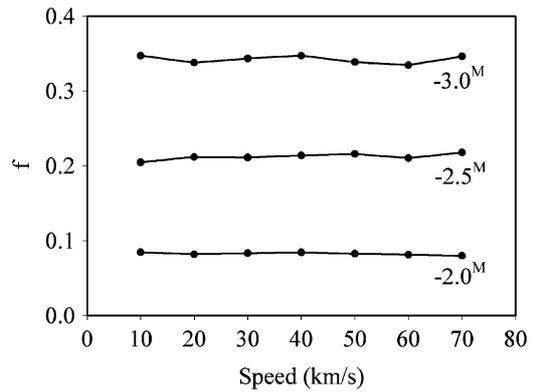
Fig. 6. Results of numerical simulation for determining likely error in speed as a function of speed and magnitude of the train relative to that which is just detectable at the main station.
