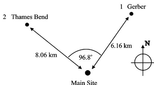
Fig. 8. Details of the UHF links between the main and remote sites.
