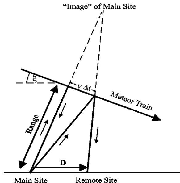
Fig. 1. Geometry of reflections on main and remote stations.
