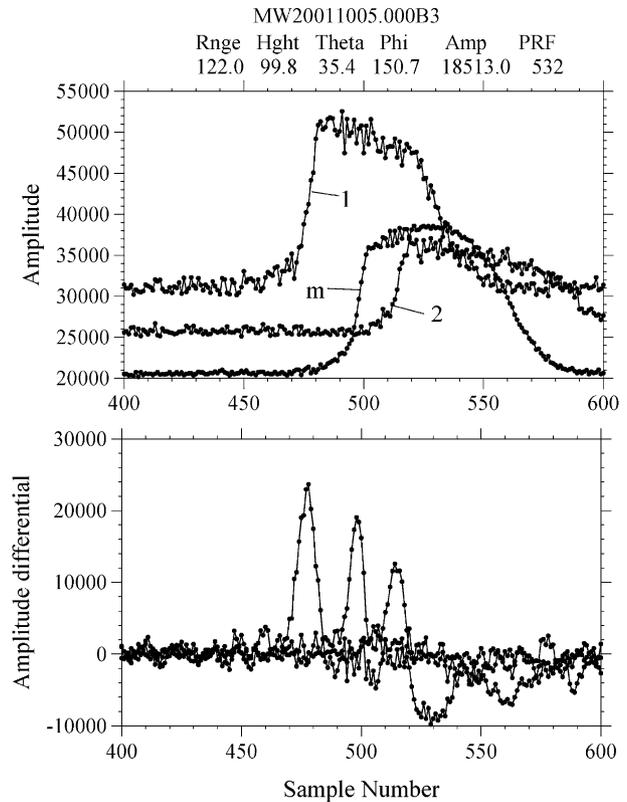
Fig. 9. Example of the (a) echo profiles and (b) the time differentials of the echo profiles received at the main (m) and remote stations.
