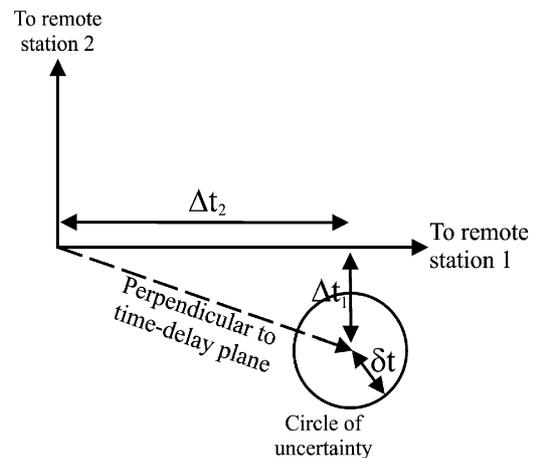
Fig. 10. The uncertainty in the orientation of the vertical time-of-flight plane is determined by the errors in the measurement of delay times of the echoes received at the remote stations relative to the instant at which the echo arrives at the main station.
