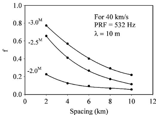
Fig. 4. Results of numerical simulation for determining fraction of meteors detected at the main site that yield orbits as a function of distance of remote stations from the main site and magnitude of the train relative to that which is just detectable at the main station.
