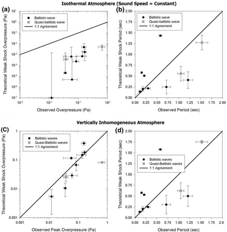
**Fig. 2** Comparison of cylindrical weak shock theory of meteor generated infrasound (ReVelle 1974, 1976) with the observations of ballistic and quasi-ballistic infrasound at ELFO for those meteors with known trajectories. **(a/b)** For an isothermal atmosphere and **(c/d)** vertically inhomogeneous (layered) atmosphere
